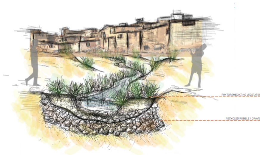
Fig. 14 - Goal of bioswales and section view.
