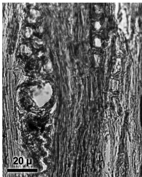
Fig. 4 - Tangential section: the rays are uniseriate, with the exception of those enclosing resin canals which are biseriata.
