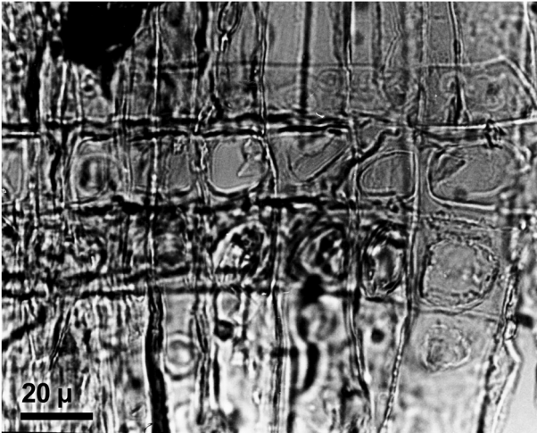
Fig. 6 - Radial section: cross-fields with pits pinoid type in the early wood and in the shape of an oblique fissure in the late wood.
